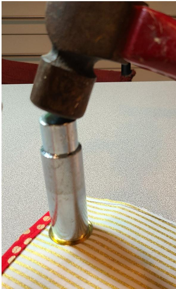
Also– I generally tilt the tool a bit in several areas and hit it with the hammer on the circular edge, just to make sure the raised of the grommet underneath gets “rolled back” well.
