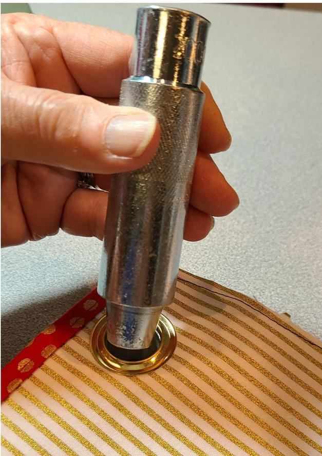
Now insert the other part of the Grommet tool into the opening and then using a hammer, Hit the top part of the tool several times quite hard to bend that raised section of the grommet so it will hold in place
