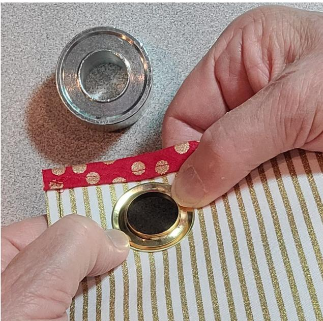
While holding both pieces of the Grommet firmly together, Place it EXTERIOR side DOWN into the Grommet tool.
