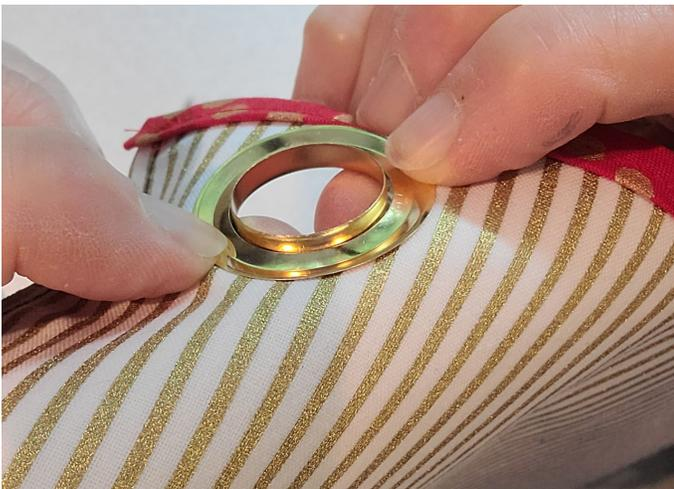
Now place the inner Grommet piece over the raised edge of the outer piece so that the curved inside area of it nestles down INTO the curved inside area of the outer Grommet.
