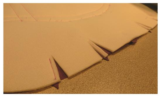
Flip Front & Back units ESD on flat surface. *Carefully* cut away six triangles of <u>foam</u> (~1" tall X 1/4" wide) along bottom edge of both units as follows:
