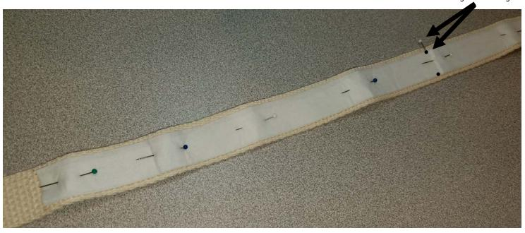
Center interfacing on webbing aligning midpoint marks then baste it in place along both long edges.
