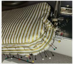
I find it easiest to start stitching a FULL 1/4" from edges at the top of the Wall/Expander (just under the area I left open & unpinned above).
