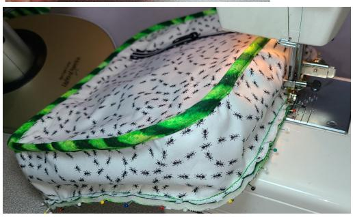
Stitch a scant 1/4" from edges with "zippered" side of Center Wall face DOWN on machine bed. Restitch entire seam for security.
