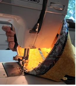
Step 35-37- Stitching in this way looks a little awkward doesn't it, and you know what? It IS a little askward, but its WAY easier than trying to stitch it together with the Bag Bottom face down on the machine bed.
